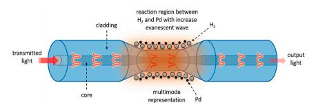
Figure 7. Hydrogen-palladium sensing mechanism.
