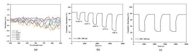
**Figure 5.** (a) Absorbance versus optical wavelength, (b) dynamic absorbance curves, and (c) repeatability of Pd-coated sensor.
