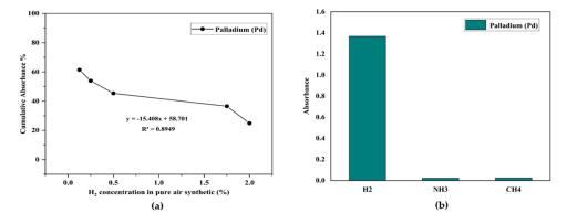
**Figure 6.** (a) Absorbance changes at different H<sub>2</sub> concentrations for Pd-coated sensors and (b) the selectivity of the Pd-coated sensor.
