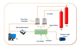
Figure 2. The experimental setup of the H<sub>2</sub> sensor.
